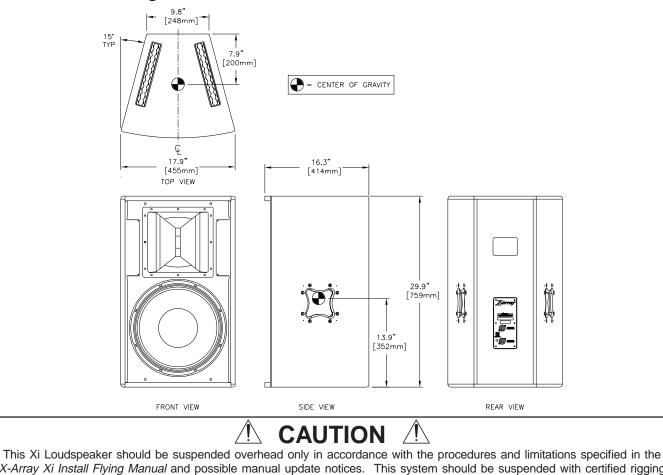
X-Array Xi Install Flying Manual and possible manual update notices. This system should be suspended with certified rigging hardware by an authorized rigging professional and in compliance with local, state, and federal overhead suspension ordinances.
